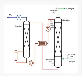
Figure 1: Sketch of a typical carbon dioxide capture plant
