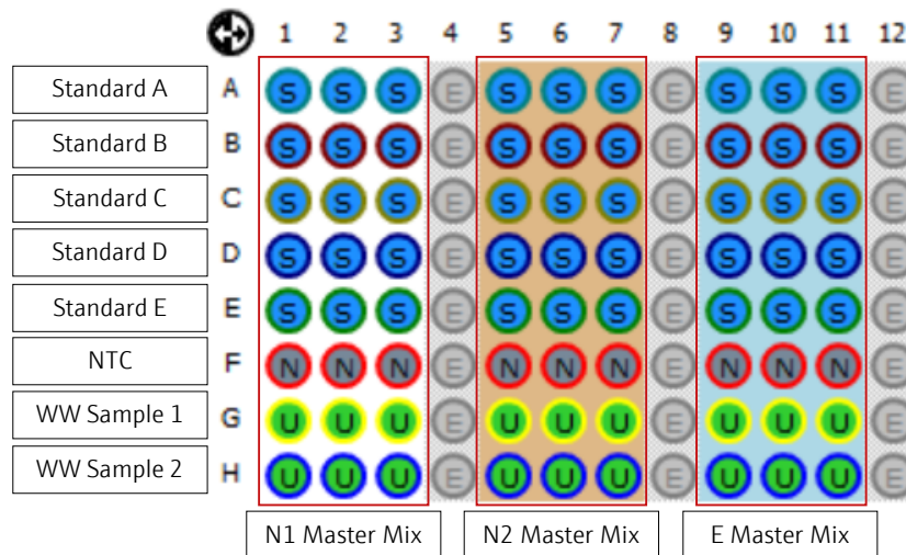
Figure 1. PCR plate map combining all three available assays and with two WW samples. All reactions were performed in triplicate.
