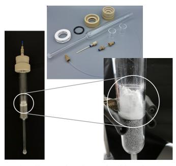
A salt crucible protects the combustion tube and the catalyst
