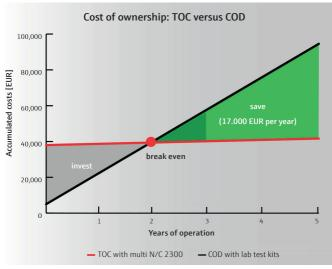
Accumulated costs of 70 samples per week using a multi N/C 2300 TOC analyzer vs. COD lab test kits. TOC analysis carried out as duplicates, COD as single analysis.
